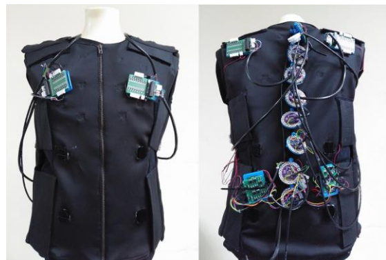
Fig.1. Haptic Vest seen from front (left) and rear (right). The hardware control (microcontrollers, PCBs and power supply system) is strategically located at the back to make easier the user movements.
